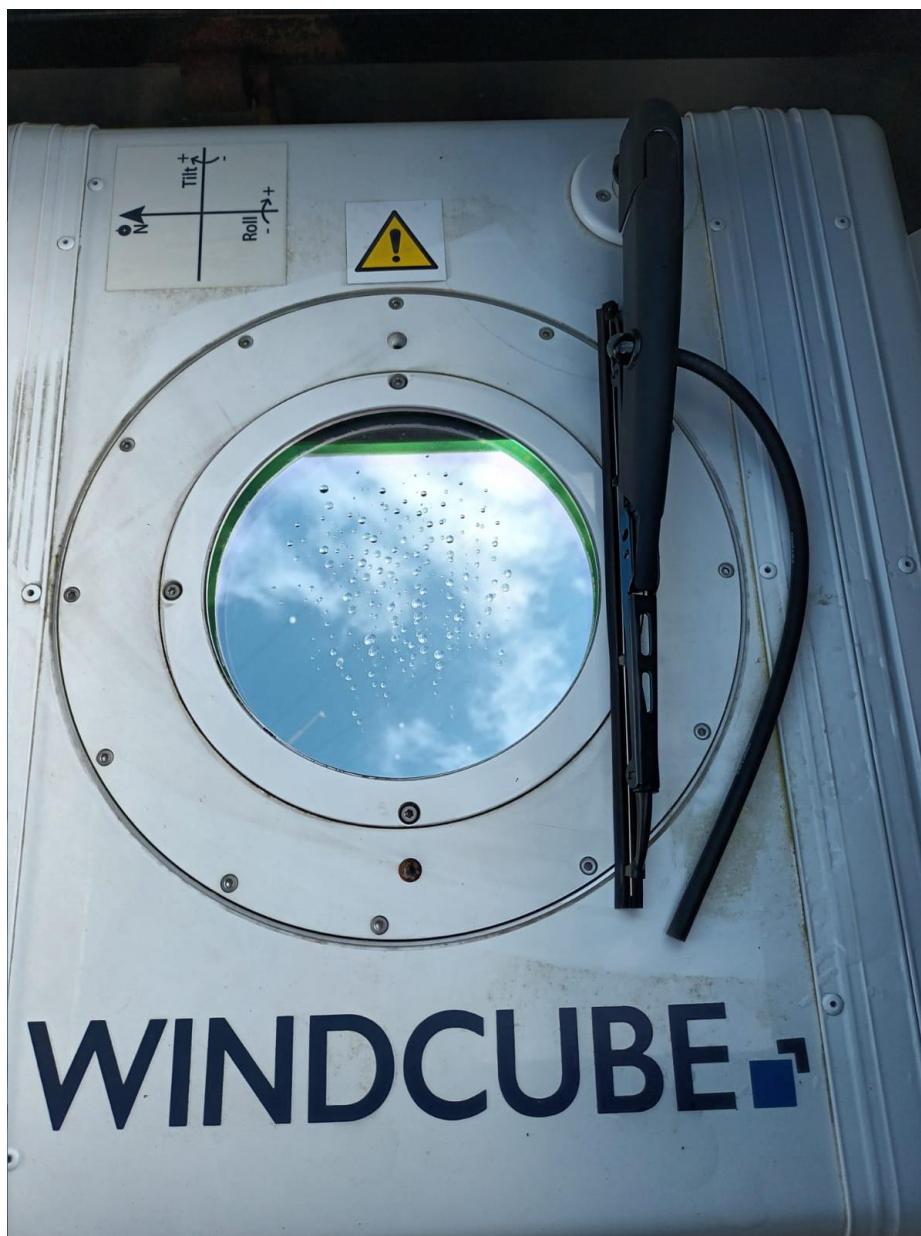
Figure A: Wind Monitoring Equipment (WindCube), Photographed at Lemanaghan Bog. The above image shows a WindCube wind monitoring device photographed within Lemanaghan Bog. This equipment is used to collect wind-related data and may form part of the assessment process informing proposed wind energy development. Clarification is respectfully requested as to whether data collected from this equipment, together with any associated wind measurement mast(s) within Lemanaghan, has been included within the planning application documentation and made available for public review and comment. Given the significance of this information in informing the proposed development, the public should have the opportunity to fully examine and consider any such data as part of the planning process.
